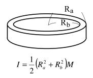
Now, measure  $R_a$  and  $R_b$ , then calculate the above moment of inertia.
