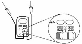
When measuring a current, select the mode indicated by the symbol 'A.'
