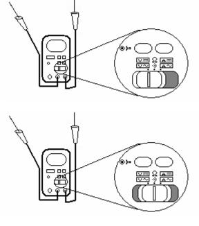
When measuring a voltage, select the mode indicated by the symbol 'V.'
