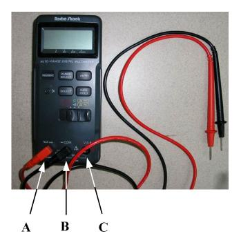
There are two kinds of power supplies to be measured by a multimeter. One is DC (Direct Current), and the other is AC (Alternate Current). In each case, you have to select the proper mode in the multimeter. When you measure the DC, you have to select to have indication, , on the window. When you measure the AC, you have to select to have this,  $\checkmark$ , on the window.
