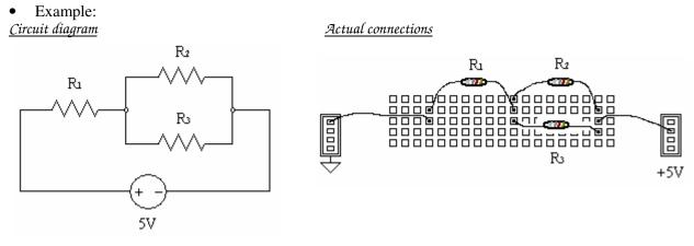
• Make the following circuit. (Draw the connections.) <u>Circuit diagram</u> <u>Actual connections</u>
