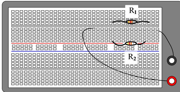
② Measure the current going through  $R_2$ . ① The following circuit is **incomplete!** **Draw the wiring and sensors first, and then implement circuit on the board.** . (Hint: Pull out the wire, which is going to the ground, from the breadboard. Then, connect the probes of a current sensor or a multimeter in series, namely, between one wire of  $R_2$  and the ground.)
