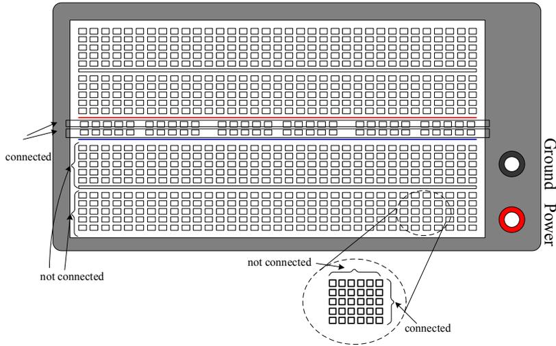
This is called a breadboard. There are one power connection and one ground. As you can see, five holes consist of one unit. These are connected and a different unit is disconnected from the other.
