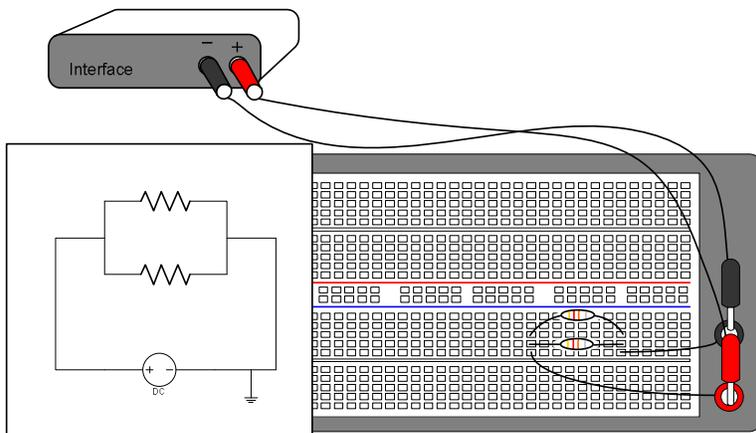
This is a parallel connection of two resistors.
