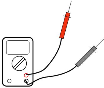
⇨ A multimeter looks like the figure. This can measure a voltage, a current, and a resistance.
