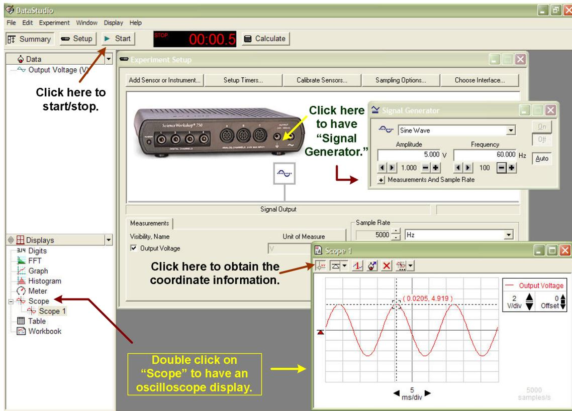
② Select “Sine Wave” (AC voltage) from the signal generator. Try following conditions. Draw the pictures by looking at what the scope shows.
