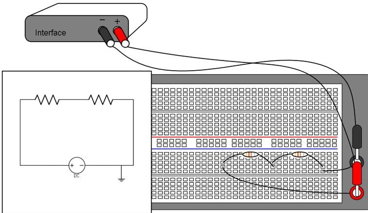
This is a series connection of two resistors. Check out which hole each terminal is plugged in.
