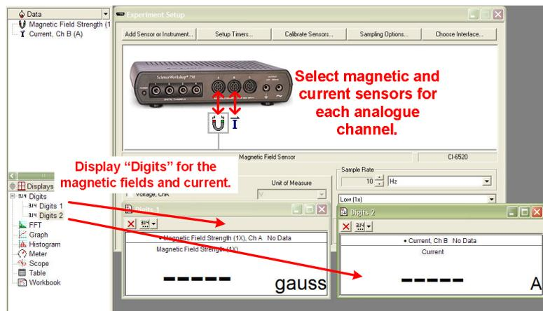
Set up the experiment as follows. Try two different orientations of the current flow: [Note that the positive magnetic field indicates that the field comes into the sensor; and the negative has to be the opposite. The current is from the positive to negative voltages.]
