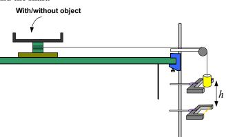
The hanging mass is fixed as 0.2 kg (200 g). <u>The initial point must be as close to the first gate as possible before the release.</u>
